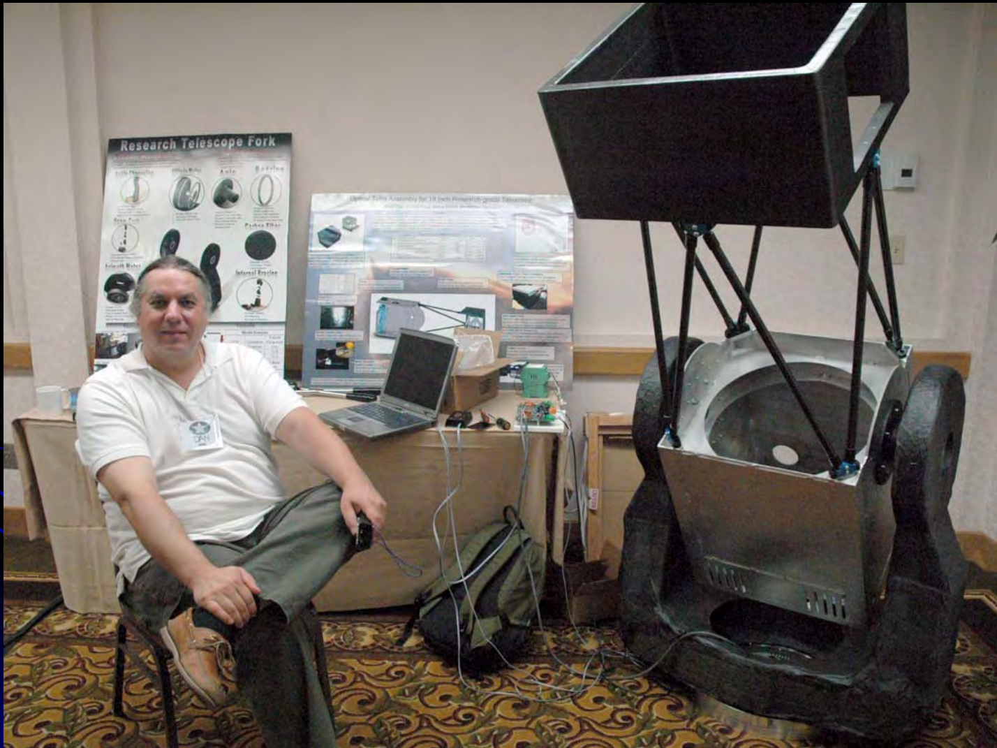
Dan Gray (SciTech) with Cal Poly fork sitting on azimuth axis motor
