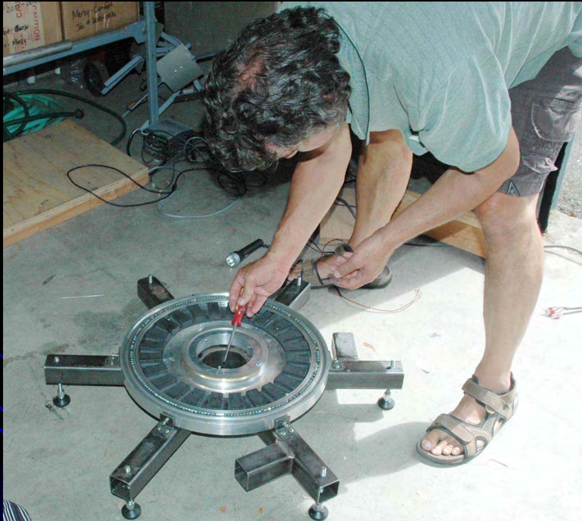
Renishaw encoder tape wraps \sim 350^\circ in azimuth
